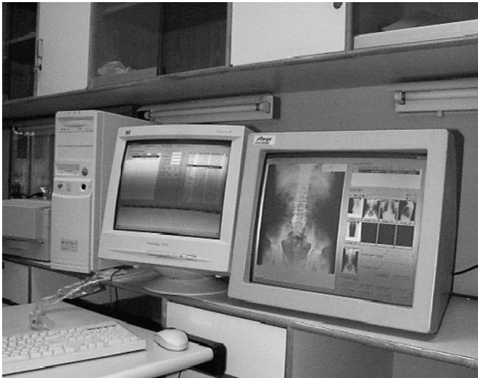
Fig. 5. Dual-monitors user interface for high-quality image display. Right side is a high-illuminate monitor; left side is an SVGA monitor.
