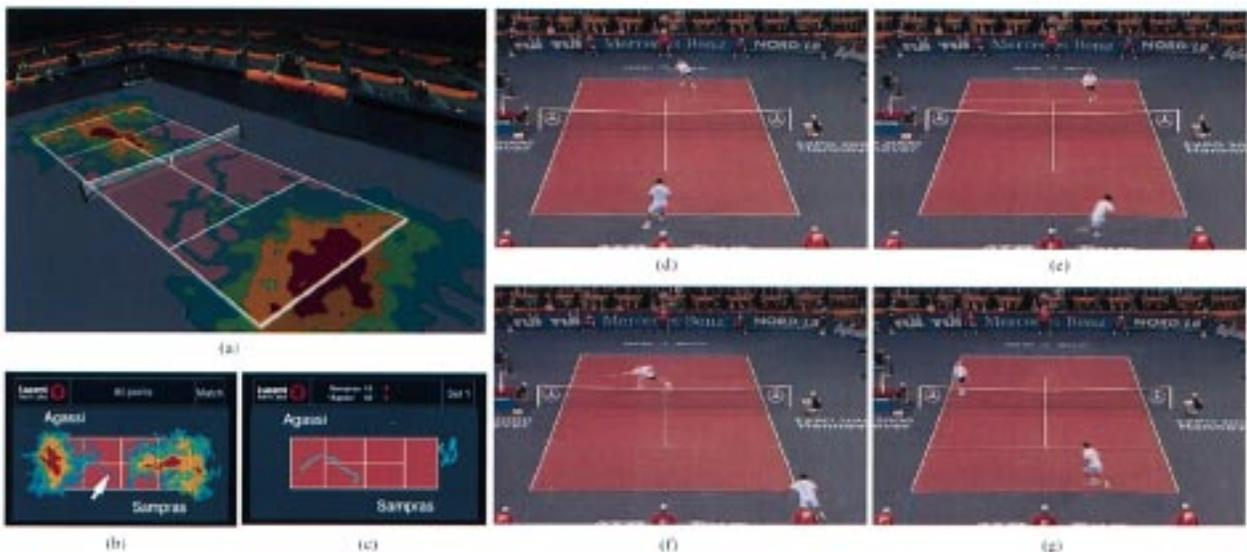
Fig. 19. Retrieving video for a particular trajectory. (a) Spatial coverage map for both players for the entire match. (b) Map viewed top down, with arrow indicating the user's selection of a portion of the map. (c) Trajectories of each player score corresponding to user's selection. (d)–(g) Four frames from the retrieved video clip corresponding to user's selection, shown clockwise.
