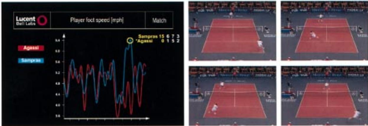
Fig. 18. Retrieving video for fastest action. Left: speed map of two players and user's selection of a portion of the map. (Speed charts were derived by video analysis.) Right: four frames from the retrieved video clip.
