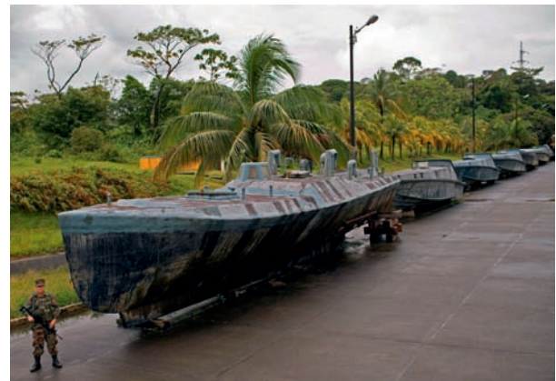
A Colombian soldier stands next to a number of 33-foot-long semi-submersible vessels captured off the coast of Colombia in 2007. Because they leave very small wakes, the crude subs are difficult to detect visually from the air or by radar.
