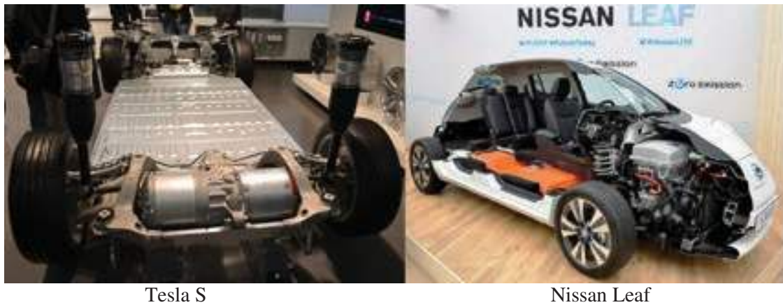
Figure 3. Comparison of Tesla S and Nissan Leaf
